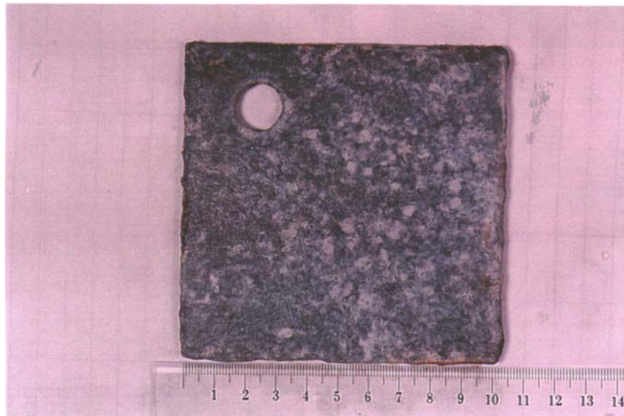
Picture 4 The surface appearance of the sample with serial number 8 after the 1000 hours salt spray test.
