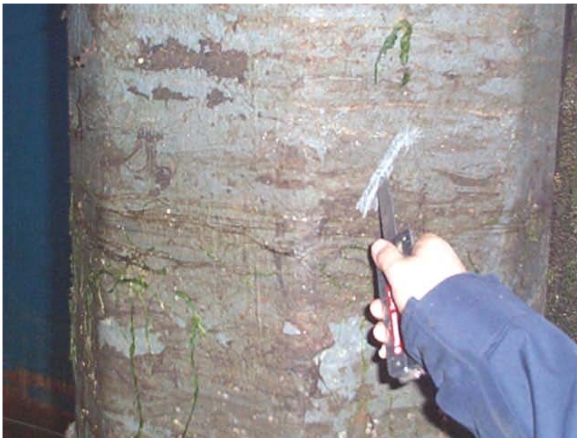
Plate 2. Testing for hardness and bounding of the coating to steel.
